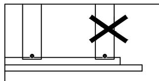
Note: Do not lock the screws of the bed slats to the outermost edge of the bed slats, you need to leave a certain space at the edges, otherwise it will cause the board to break.
