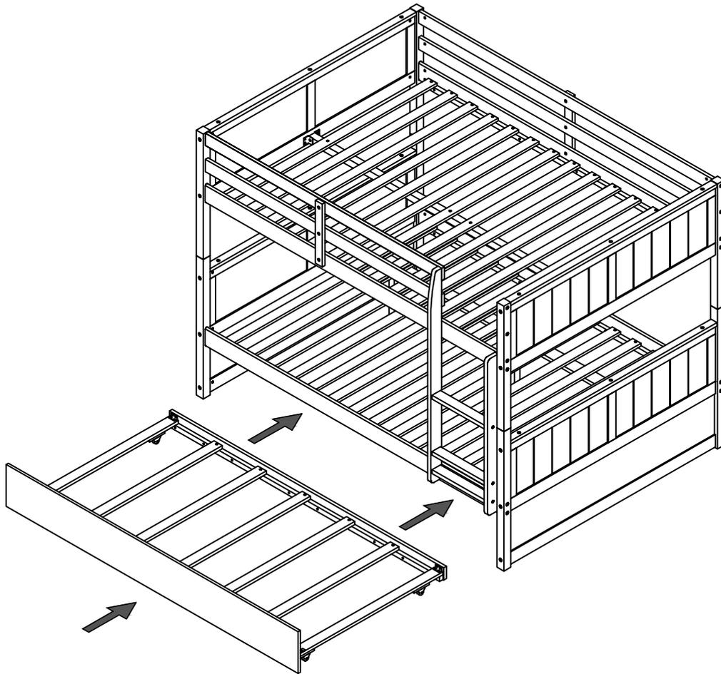
Push Trundle under the bottom of Bunkbed.
