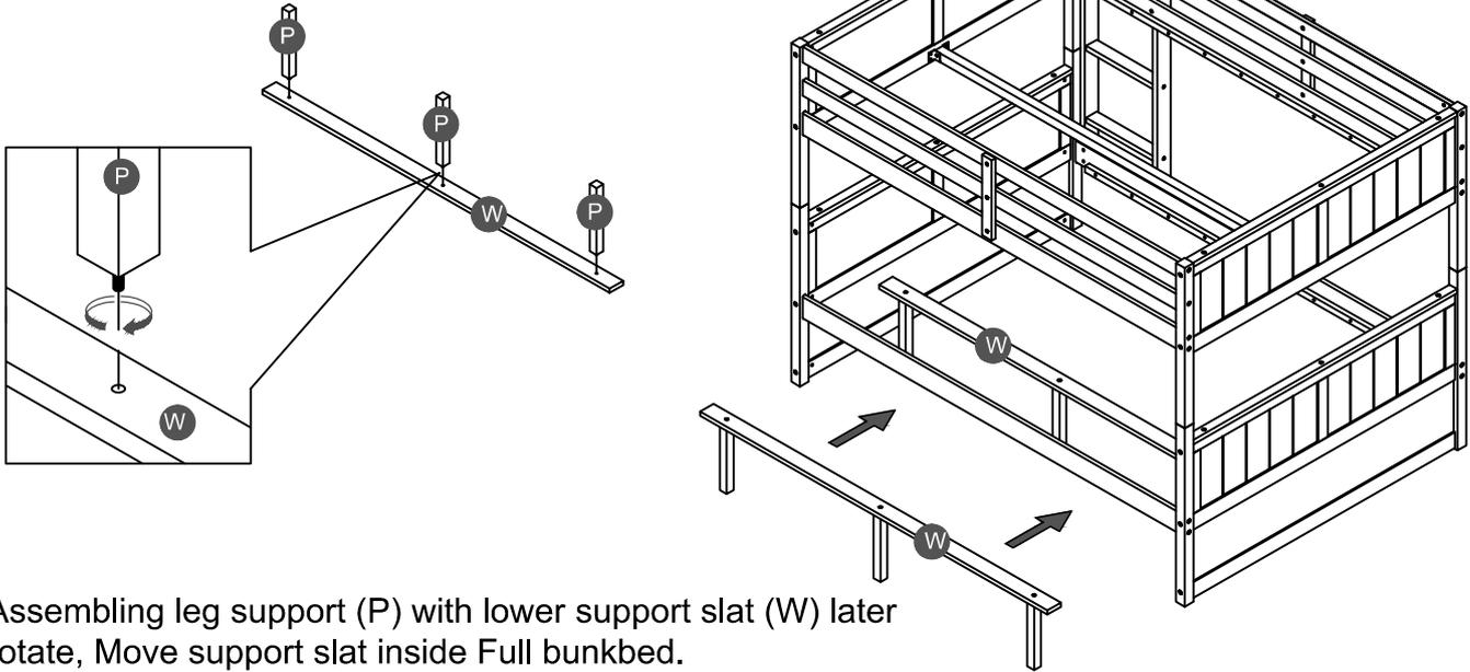
Assembling leg support (P) with lower support slat (W) later rotate, Move support slat inside Full bunkbed.
