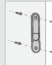
Install the cradle bracket to the wall with the included screws.
