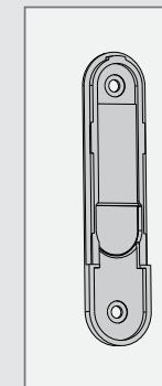
Slide the cradle onto the mounted bracket.
