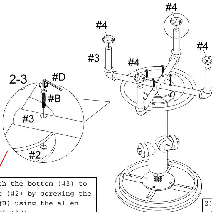
3) Attach the bottom (#3) to the base (#2) by screwing the bolts (#B) using the allen wrench M5 (#D).
