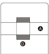
Please ensure threaded cylinders (#D) are popping out on each ends of panel (#A) by approximately 0.3 inches so there is enough threading on each ends of panel (#A) to secure poles.
