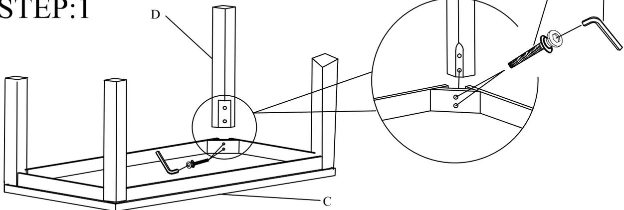
Step 1. Lay table top on a flat soft surface with the table top facing down, make sure no bolts or any sharp objects are underneath. Align table leg with the holes on each corner and bolt on the bolts. Place all bolts in without tightening all of them until all four legs are placed in . Once all are tightened carefully flip the table over with two or more people . We hope you enjoy this table !
