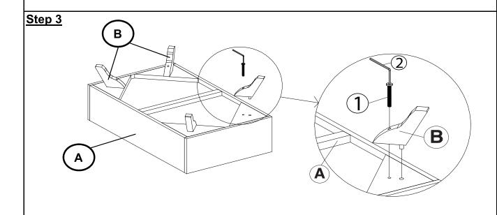
Repeat the same process as Step 2 to affix 3 remaining Legs (B) with the Bed (A). **DO NOT FULLY TIGHTHEN THE BOLTS**
