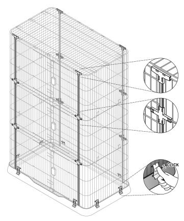
To solidify the entire cage, press a connector onto each panel intersection until it clicks and all surfaces are flush.
