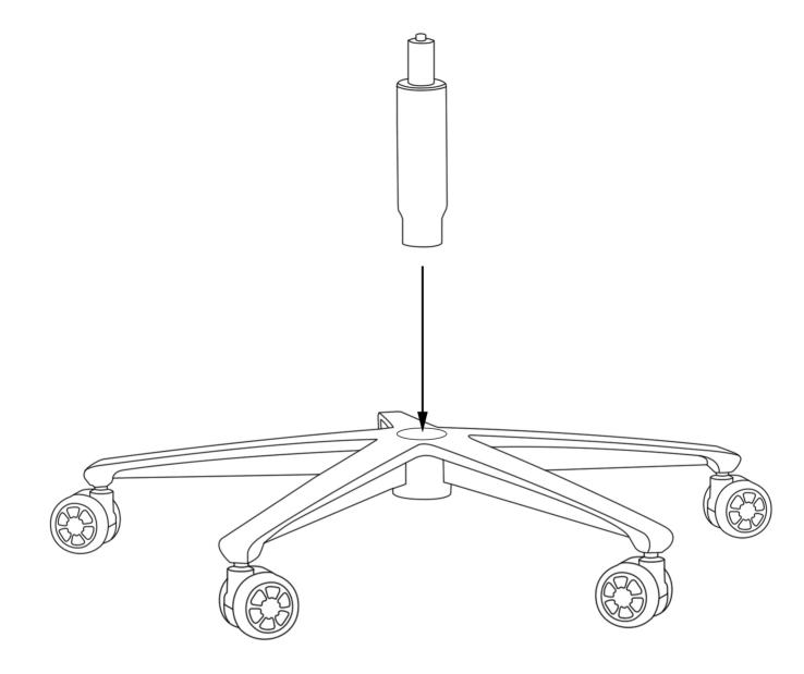
2.INSERT THE GAS LIFT INTO THE CENTER HOLE OF THE STAR BASE.
