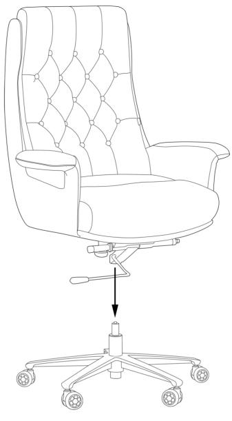
4. LAY THE ASSEMBLED CHAIR BODY ON ITS SIDE, TAKE THE STAR BASE, AND AFTER INSERTING THE GAS LIFT INTO THE CENTER HOLE OF THE SEAT PLATE, STAND THE CHAIR UPRIGHT TO COMPLETE THE INSTALLATION.
