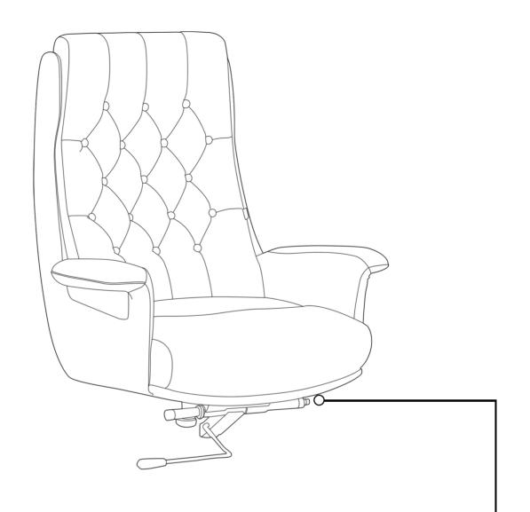
3. ALIGN THE SEAT PLATE WITH THE PRE-DRILLED HOLES BENEATH THE CHAIR BODY ENSURING THAT THE FRONT END OF THE SEAT PLATE FACES THE FRONT END OF THE CHAIR BODY SECURE THE SEAT PLATE TO THE CUSHION USING FOUR BOLTS. TIGHTEN ALL THE BOLTS WITH A WRENCH.
