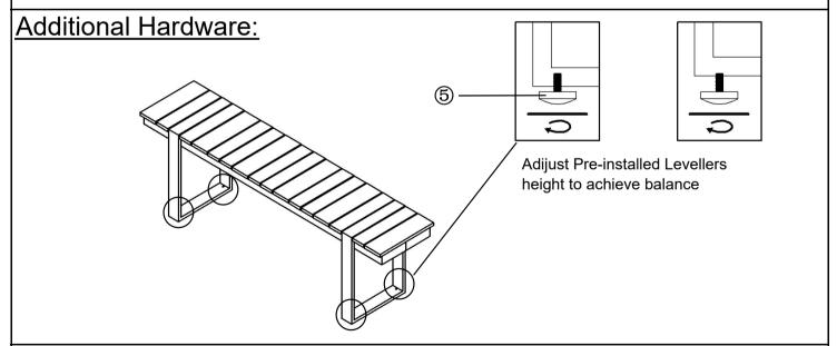
Insert the adjusting foot pad (⑤) into the Leg tube(A), as shown in the figure above.
