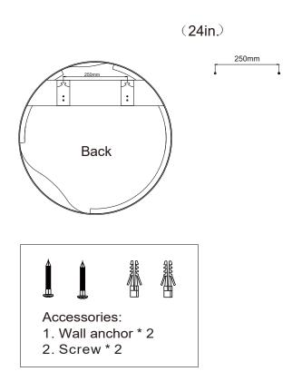
1.Punch 2 holes in the wall with an electric drill at the proper height, leaving a hole spacing of 250mm.
