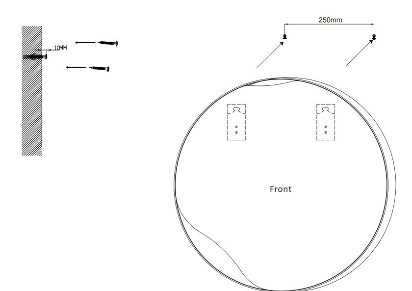
3.Make sure to leave a 10mm gap between the screw head and the wall.
