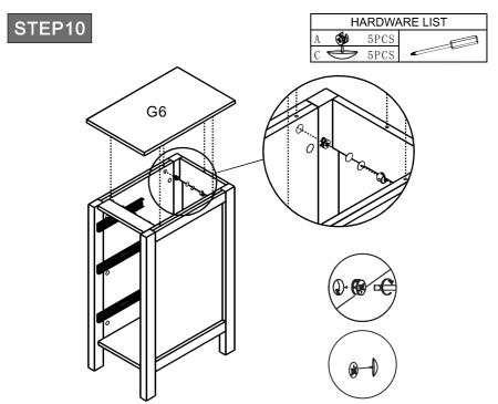
• Insert shelvesG6 downwards to their corresponding positions, then tighten the cam lock.
