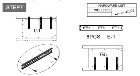
• Insert the screws to connect the slides (E-1) to the shelves.
