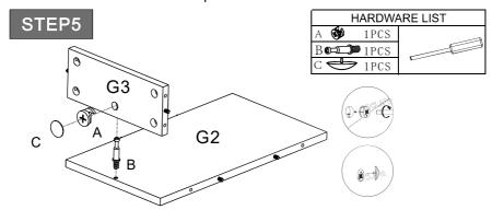
• Insert shelves G2 and G3 downwards to their corresponding positions. then tighten the cam lock with the cover.
