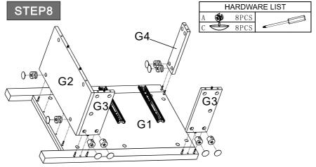
• Insert shelves G1,G2 and G3 downwards to their corresponding positions, then tighten the cam lock.
