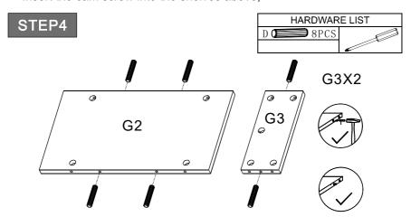
• Insert the wooden dowel pins into the shelves.
