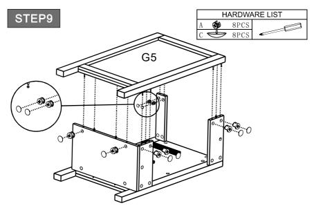
• Insert shelvesG5 downwards to their corresponding positions, then tighten the cam lock.
