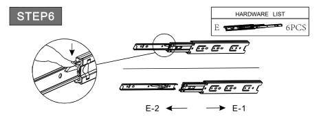
• Press the button and extend the slide slowly. Then separate it with the release latch. Repeat these steps for the other slides.
