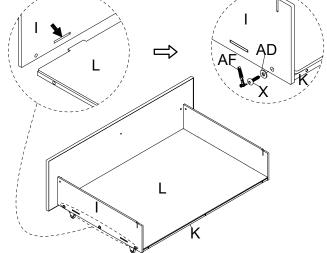
Attach the Drawer Back Board (J) to the Drawer Bottom Frame (K), insert the Bolt (X) and Washer (AD), turn the Ratchet Tool (AF) to tighten them. Attach the Drawer Board Connector (Q) to the assembled drawer, insert them into correct places.
