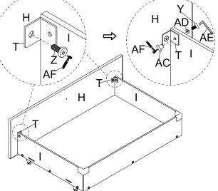
14 Insert the Bolt (AA) and Washer (AD) to the back of Drawer Front Board (H), turn the Ratchet Tool (AF) to tighten them.
