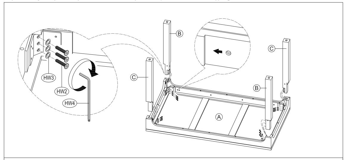
STEP 1 ATTACH LEGS 1 (B) AND LEGS 2 (C) TO TOP ASSEMBLY USING BOLTS 30 MM (HW2) AND SPRING WASHERS (HW3). TIGHTEN THE BOLTS USING ALLEN KEY (HW4).
