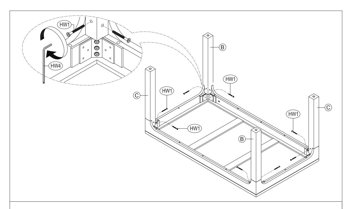
STEP 2 ATTACH BOLTS 60 MM (HW1) TO LEGS 1 (B) AND LEGS 2 (C). TIGHTEN THE BOLTS USING ALLEN KEY (HW4).
