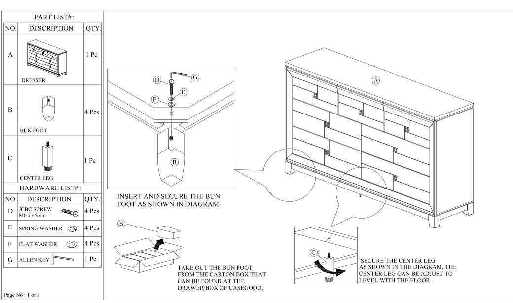
NOTE: SCREWS WILL BECOME LOOSE WITH USE AND OVER TIME WILL NEED TO BE TIGHTENED PERIODICALLY. CHECK TIGHTENESS OF SCREWS EVERY 6-8 WEEKS. THANK YOU FOR PURCHASING THIS QUALITY PRODUCT. BE SURE TO CHECK ALL PACKING MATERIAL CAREFULLY FOR SMALL PARTS WHICH MAY HAVE BECOME LOOSE INSIDE THE CARTON DURING SHIPMENT.
