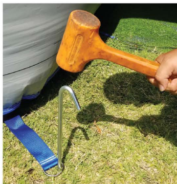
2. Drive the stakes down in a 90 degree angle through the D-Rings. Be sure not to hit any utility lines.
