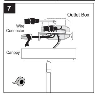
Carefully arrange excess wiring and wire connectors within canopy.
