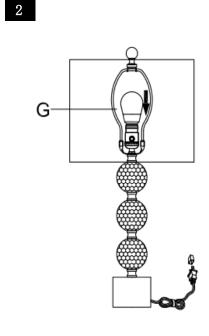
Step2 Insert the bulb(G) into the socket(C).
