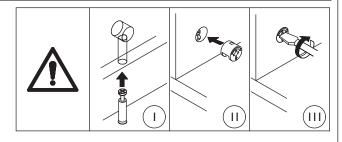
Attach another plate 7 and 8 to plate 5, add cam lock(B) into plate 7, 8 and turn clockwise to tighten as shown.
