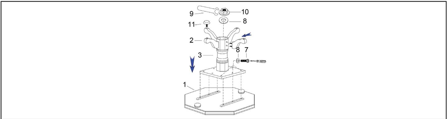
4. Carefully turn table over. Place TABLE TOP #5 on top of assembled TABLE.
