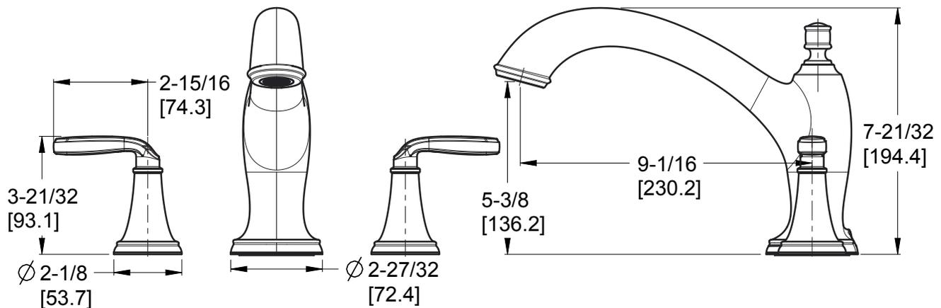
$\varnothing 1$  Min to  $\varnothing 1\frac{1}{2}$  Max. Deck Hole Openings
