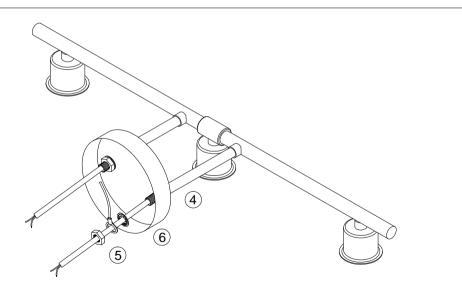
3.Install the fixture with canopy ⑥ together with nuts ⑤ (note the earth wire should between two nuts).
