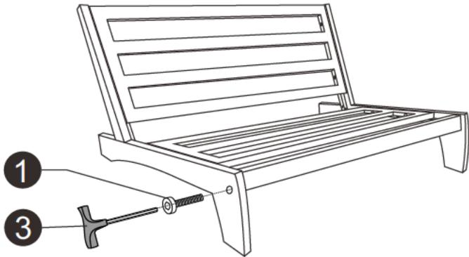
**STEP 8:** Fix the left end of stretcher with bolt(1) and allen key(3).
