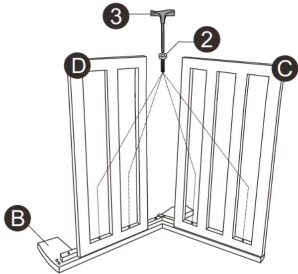
**STEP 4:** Connect seat frame and back frame to right legs with bolt(2) and allen key(3).
