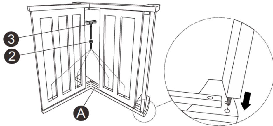
**STEP 7 :** Place frame (step 6) to left legs( A), fix with bolt (2) and allen key (3).
