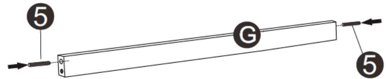
**STEP3:** Insert wood dowel(5) into holes at both ends of stretcher(G).
