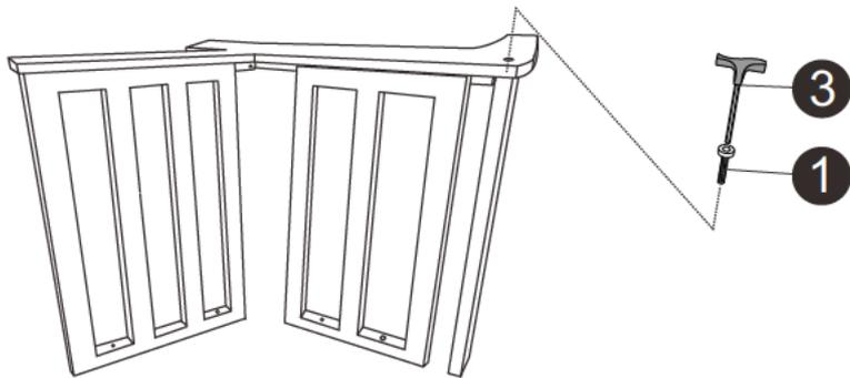
**STEP 6:** Invert the frame (step 4), fix the stretcher with bolt(1) and allen key(3).
