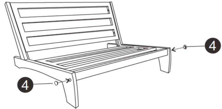
**STEP 9:** Cover the screw holes on both sides of legs with plastic cover (4).
