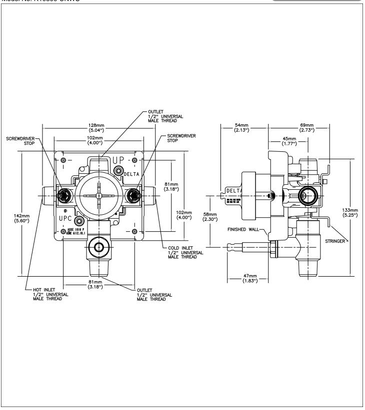
Delta reserves the right (1) to make changes to specifications and materials, and (2) to change or discontinue models, both without notice or obligation. Dimensions are for reference. Measurement may vary plus or minus 6mm(0.25"). Mounting locations are suggested only. Check with local codes for requirements in your area. This spec was produced September 03, 2015.
