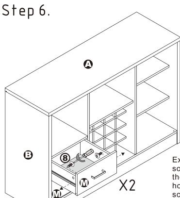
Extend the two outer slides of the runners so that they could align with the sides of the drawer. Make sure the pre-drilled holes from the drawer align with the screw holes of the outer slides.
