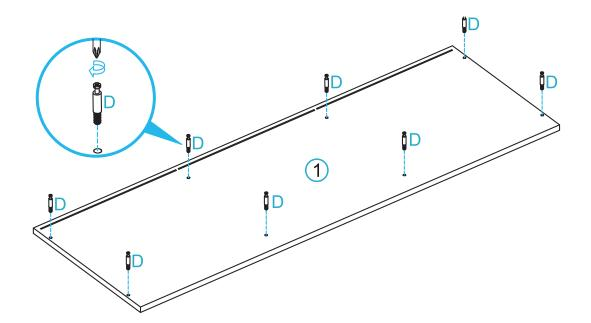
Attach 8 x bolts (D) to panel [1]. Tighten with a screwdriver.
