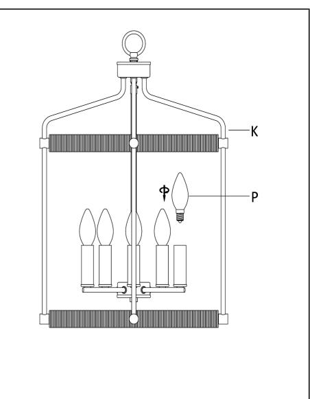
**Step 6:** Insert the bulbs (P) into the Sockets
