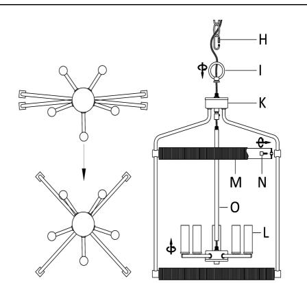
**Step 2:** The Lamp Body (K) hit flat pipe to adjust, Rotate the Tube (O) clockwise to secure it to the Lamp Body (K), clockwise rotation Socket (L) to fix it to the center of the Lamp Body (K), clockwise rotation Cylinder (N) to fix the Circle (M) to the Lamp Body (K) on the bend, Thread Fixture Loop (I) to Lamp Body (K) of the nipple. Attach the Closable Link (H) onto the Fixture Loop (I).
