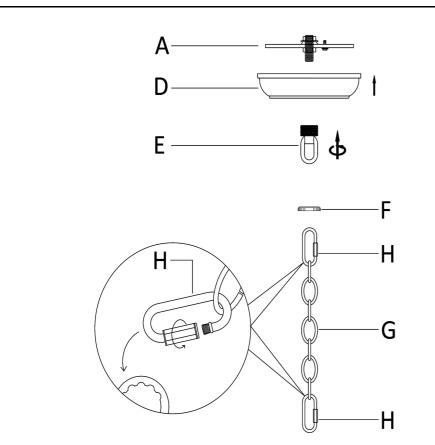
**Step 1:** Unpack all parts from cartons carefully. Place the Canopy (D) onto the Hanging Loop (E). Place the tube of the Mounting Plate (A) into the threaded portion of the Hanging Loop(E) and assemble by turning the Canopy Nut (F) clockwise till tight. Attach the Closable Link (H) onto the Hanging Loop (E)
