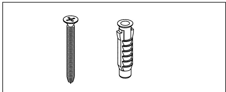
2. If it is a wooden wall (the thickness of the wooden board needs to be at least 15 mm), you need to buy automatic screws locally.
