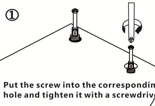
Put the screw into the corresponding hole and tighten it with a screwdriver.
