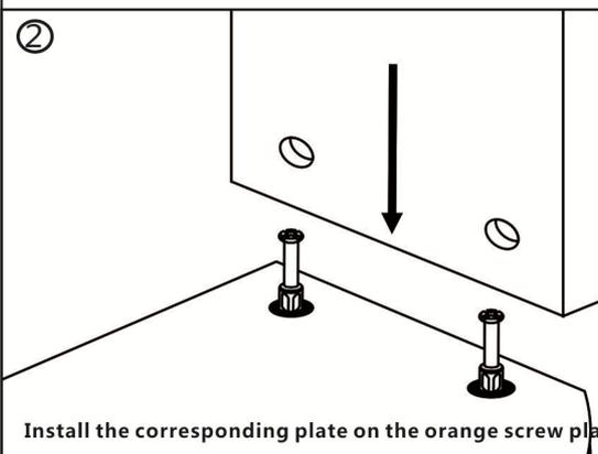
Install the corresponding plate on the orange screw plate.
