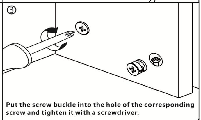
Put the screw buckle into the hole of the corresponding screw and tighten it with a screwdriver.
