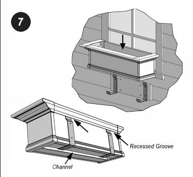
Place the window box directly over the wall mount brackets and slide straight down. The top of the brackets should slide into the recessed groove on the back panel. The front part of bracket should fit inside the channel running down the center of the bottom panel. Gently pull on the window box to make sure the brackets are seated properly.
