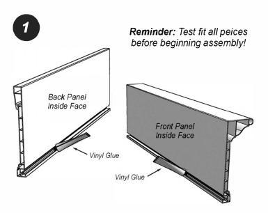
Identify the front and back panel from the part list. Run a continuous bead of glue along the groove on each panel. Be generous to ensure each groove has plenty of adhesive to create a good seal.
