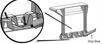
Identify the right and left end caps from the part list. Starting with only the Left End Cap, run a continuous bead of glue along the internal walls of the cap. Be generous with the glue to ensure a strong seal is formed between the panels and end cap.
