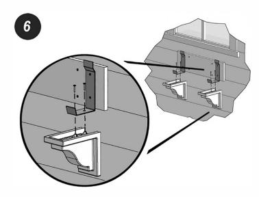
To install the optional decorative brackets align the holes with the wall mount brackets (decorative brackets are sold separately). Secure using the two screws provided with the decorative brackets. The molded vinyl brackets are decorative only so there is no need to over tighten the screws.
