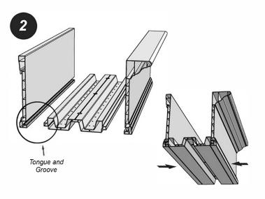
Position all 3 panels as shown above ensuring the bottom panel has the perforated holes facing up. A tonque and groove design provides easy alignment between the panels. Squeeze the parts together and check for a tight fit throughout the length of the panels. For best results clamp the panels together while the glue cures.
