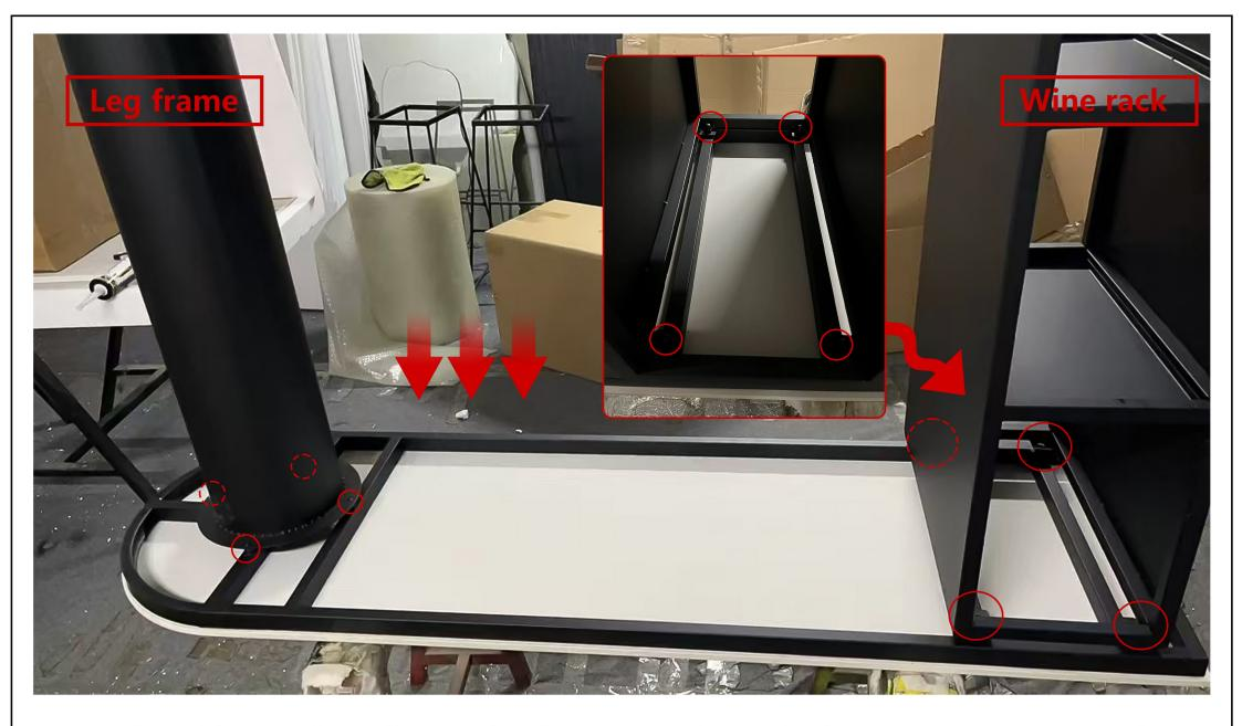
Turn the table over first, align the leg frame and wine rack with the screws on the table. The screws are installed in advance. After placing them in a good position, screw four nuts on each side to tighten and fix them. Turn the table over after installation.
