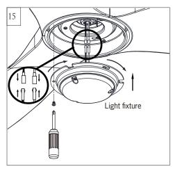
Connect white wire from fan to white wire from LED light fixture and then connect blue (or black) wire from fan to black (or blue) wire from LED light fixture. Be sure plugs connection clasped together completely. Attach LED light fixture onto the light pan, aligning the keyhole slots on the LED light fixture with the preassembled screws on the light pan. Twist clockwise till lock. Reinstall the screw removed in installation step 14. Tighten all screws securely.
