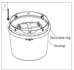
Place the decorative ring over the housing. Handle it carefully to prevent the housing gets scratch from the decorative ring. Make sure the side with grooves is upward.
