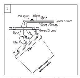
Make wiring connections as indicates above, using wire connectors provided. Connect Black wire from fan to Black (Live) wire from house. Connect White wire from Fan to White (Neutral) wire from house. Connect all green grounded wires to Grounded wire from House. Make sure that no filaments are outside of the wire connectors.
