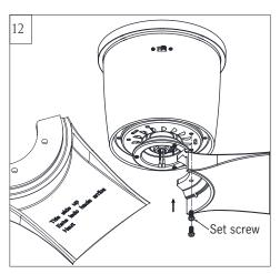
Align the holes on the blade with the screw holes on the motor. Install the blade by setting screws provided. Repeat this process for other blades. Tighten all screws securely.
