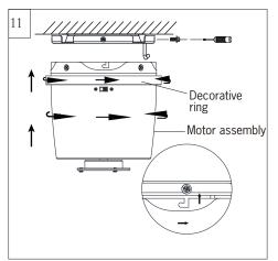
Attach motor assembly onto mounting plate, aligning the keyhole slots on the housing with the screws on mounting plate and twist clockwise till tight. Reinstall the screw removed in step 4. Tighten all screws securely. Attach decorative ring by locating the head of set screws on housing with grooves in the decorative ring and twist clockwise till tight.
