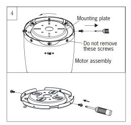
Remove the 4 set screws and remove the mounting plate from fan housing. Keep screws.
