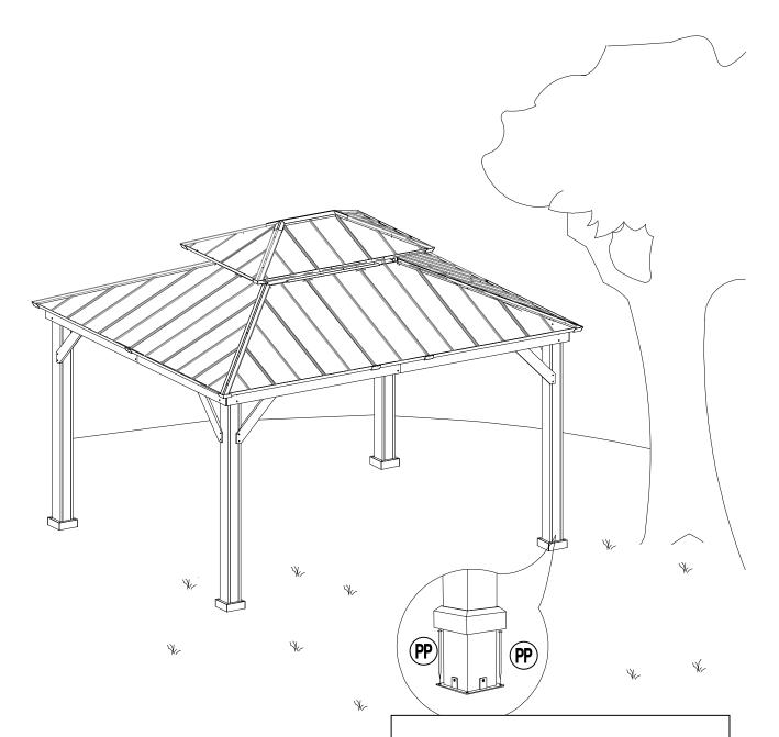
Noting: Please purchase the anchors from local hardware store if anchor the gazebo to concrete or wood. (Pls use expansion bolts to fix on the concrete ground or wooden deck.)
