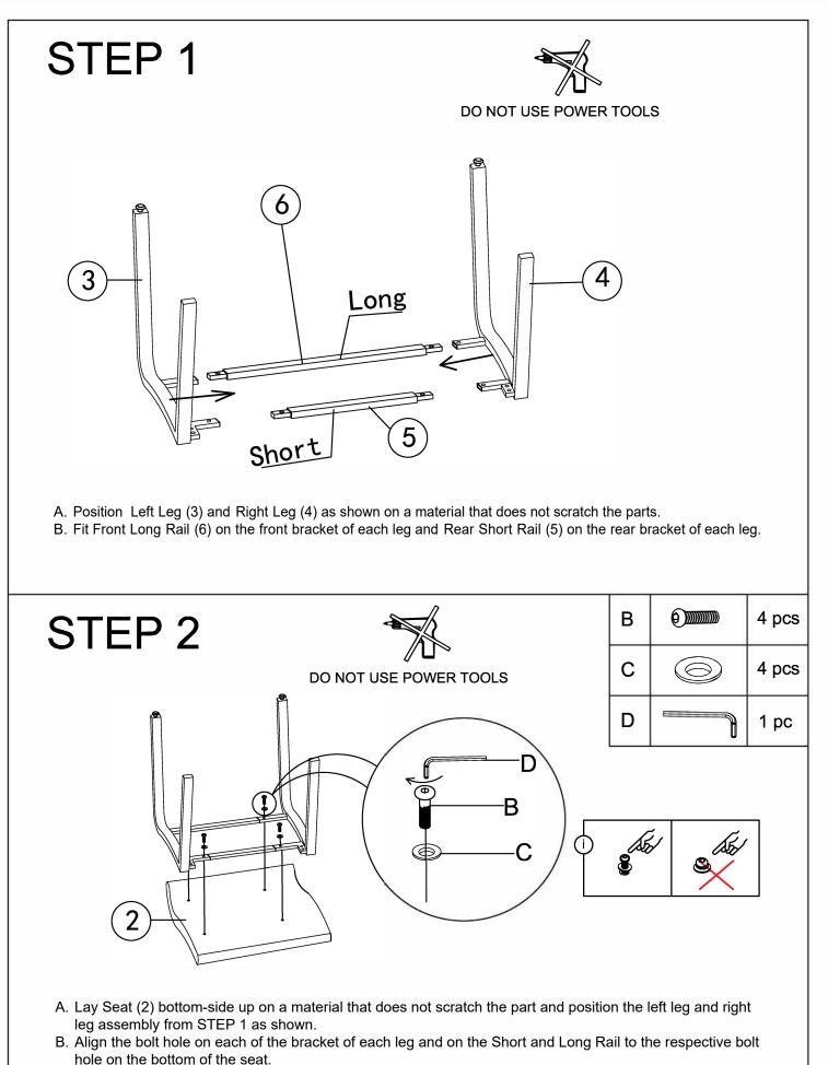
C. Use Allen Head Bolt (B) fitted with Flat Washer (C) to fasten the leg assembly to (2). Use Allen Wrench (D) to drive (B). Do not tighten (B) completely at this time.
