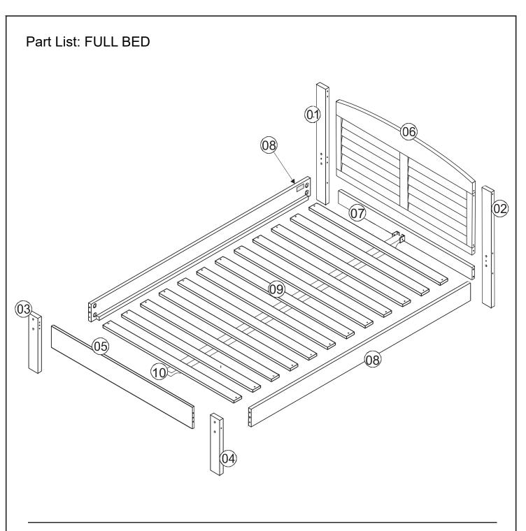
**Identifying the Hardware/part list -** Identify the hardware using the illustrations below.
