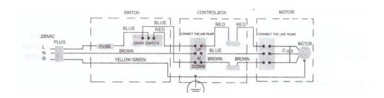
If the motorized screen work with remote control, please refer to the diagram below for electrical connection.
