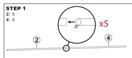
**TIP:** To avoid pinching your fingers, angle the tube with the torsion spring so the spring is on the inside the other tube, then align the tubes so they are straight and push them together.
