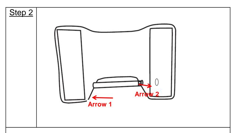
Put the Front rail(B) into the counter stool's left hole as arrow 1.
