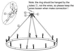
2.Let the wire go through the connected tube ©3, hang the ring ©1 to the junction box ©6 with carabiner hook screw connection @4, let the wire go through the junction box ©6.
