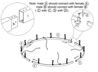
1. Assembled the split parts 1 to a completely ring fixture like picture showed, pushed the split parts and fix with bolt screw 2.
