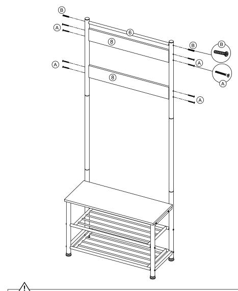
Note: During the assembly, please first half-tighten all the screws into the holes. After all the screws are set, fully tighten them.
