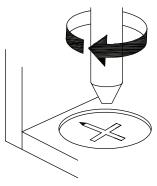
**EN**\_Turn cam lock clockwise to tighten.
