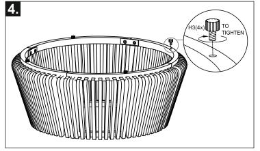
Place the base ring upside down and carefully tighten the levelers as shown above.
