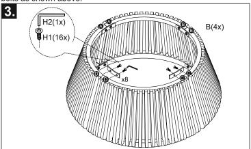
Once the ring is completed tighten all the bolts and check for any loose bolt.
