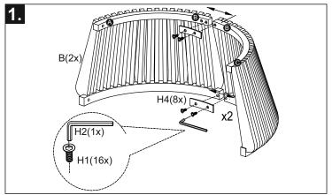
Position base segments like this & match the numbers marked on each to make a series. Place the assembly plates & tighten the bolts as shown above.
