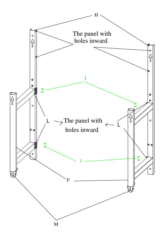
Step 4: Install E on H with 4 screw J and connect C and E with 2 screw K
