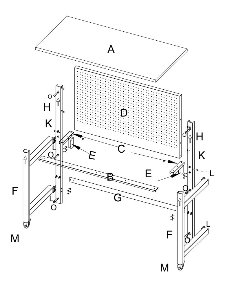
Step 1: Connect F and L with 8 screw I Step 2: Install the wheels M on F
