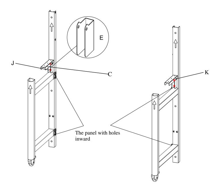
Step 5: Install G and D on H with 8 screw J and put B on F
