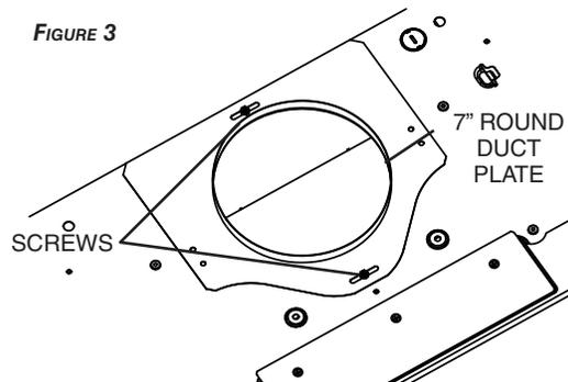
NOTE: To accommodate off-center ductwork, the 7" round duct plate can be installed up to 1/2" on either side of the hood center.
