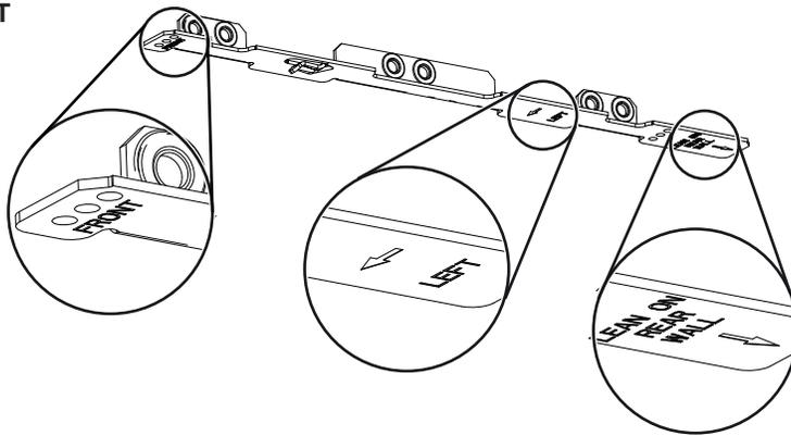
Refer to the marking on the brackets to determine the correct installation side and orientation.
