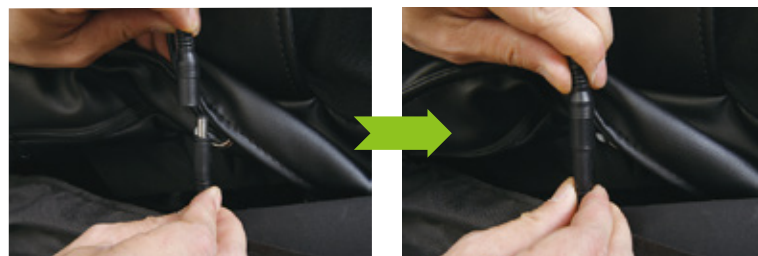
Connect back cushion heat wire.
