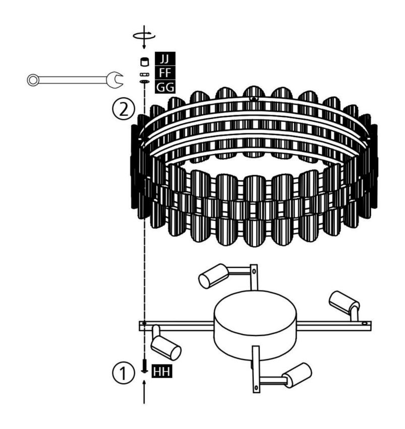
4. Remove the set screws on the fixture body
