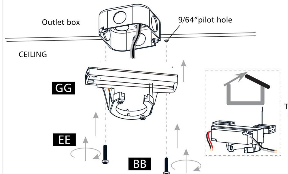
This fan cannot be used for the ceiling which angle is greater than 19 degrees.
