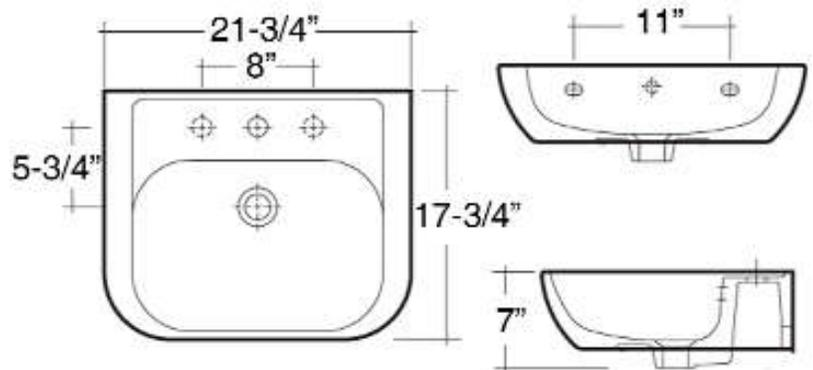
Dimensions of fixture are nominal and may vary within the range of tolerances established by ANSI Standard A112.19.2. Dimensions and specifications subject to change without notice.
