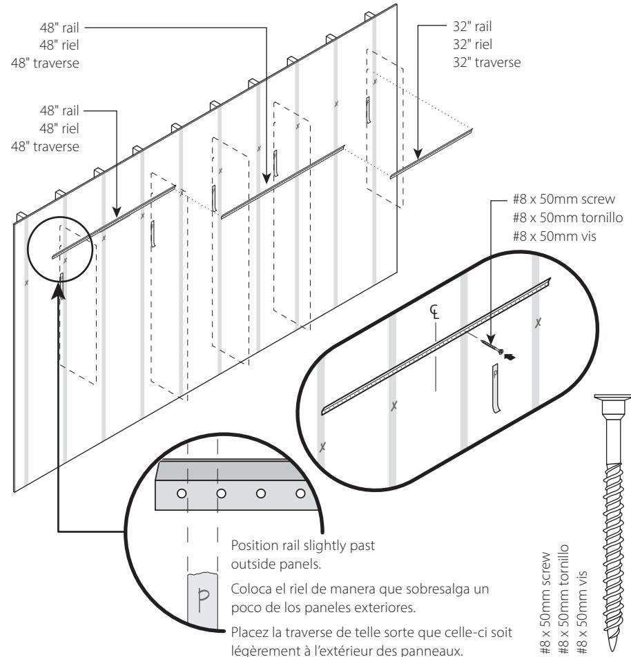
**5** Drill  $\frac{1}{8}$ " pilot holes into each stud location and in the last hole of the rail on both ends of the wall. Measure remaining rail and cut if necessary. Cut rail to correct length with a hacksaw, if necessary.
