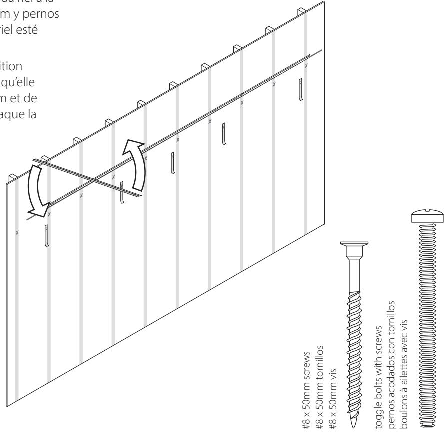
**10** Hang two (2) 48" vertical panels and three (3) 72" vertical panel onto the rail at their predetermined locations.
