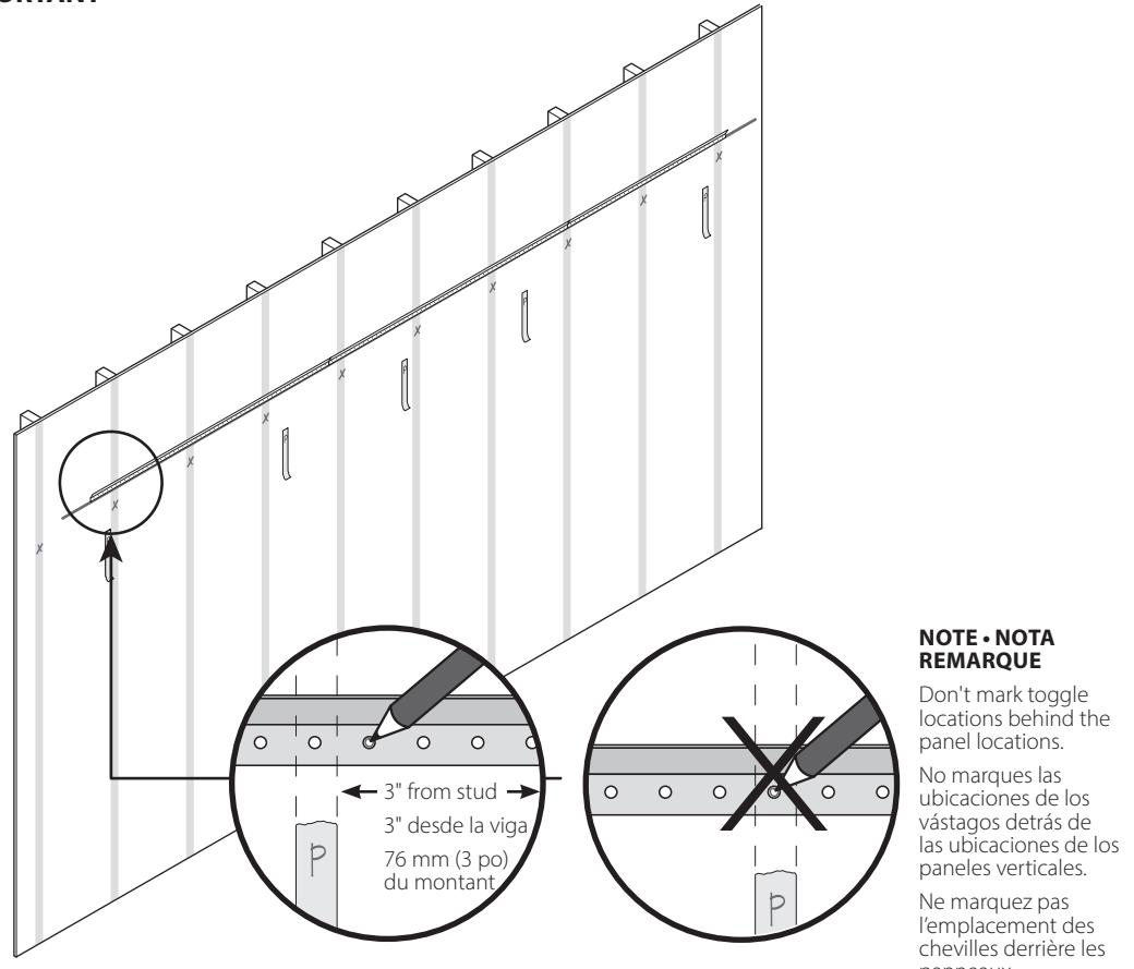
**7** Rotate rail out of position, then drill toggle holes. Use  $\frac{1}{2}$ " drill bit. Repeat for remaining rails.
