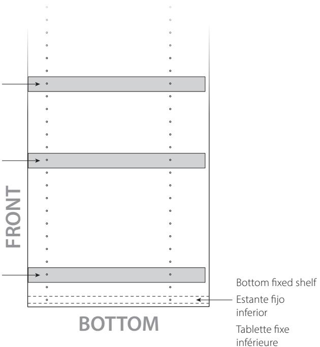
**14** Install four (4) shelf pins into verticals for each shelf. Lower adjustable shelves onto shelf pins.
