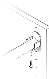
Screw rod holders to the vertical panels through the existing hole, using a #6 x  $\frac{1}{2}$ " zinc screw.
