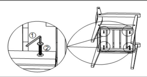
Lay down the Chair one side and Secure Seat Panel (C) with Left Panel (B2) and Right Panel (B1) by using 4 Screws (2) + Allen Key(1)
