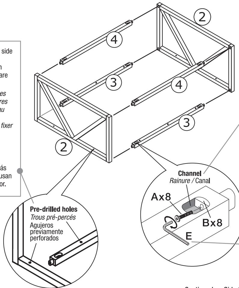
The channel on the support bars (3 / 4) need to face up during assembly.
