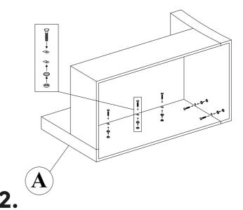
Next, attach the sofa back (A) to the sofa base and sofa side (B+C). Lay the sofa back (A) down so that the bolt brackets are facing you. Then place (B+C) in position, as shown in the above image, so that the bolt brackets are all aligned. Insert bolt (D) through the brackets of the sofa base (B) and through the bolt brackets of the sofa side (C). Then secure with a washer (F) and a nut (E). Loosely tighten the nuts and bolts with the spanner (G) and allen key (H).
