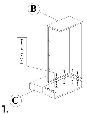
Attach side (C) to the sofa base (B). Do this by laying side (C) on the ground with the bolt brackets facing you. Then align the bolt brackets of the sofa base (C) with those in the sofa side (C) as shown in the diagram above. Insert bolt (D) through the bracket of the sofa base (B) and through the bolt bracket of the sofa side (C). Then secure with a washer (F) and a nut (E). Loosely tighten the nuts and bolts with the spanner (G) and allen key (H).
