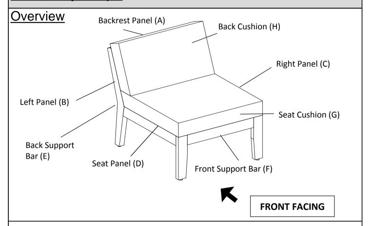
This Armless Chair has multiple parts and may require up to 30 minutes to assemble. To give you an overview of the Armless Chair parts, the above picture is to help you put the various parts into perspective. Please read through the instructions below to familiarise yourself with the parts and steps before assembly.
