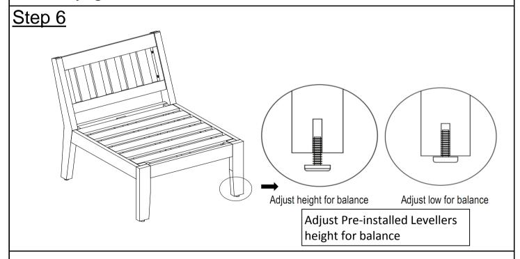
Inspect the Chair and make sure all parts are adequately connected.
