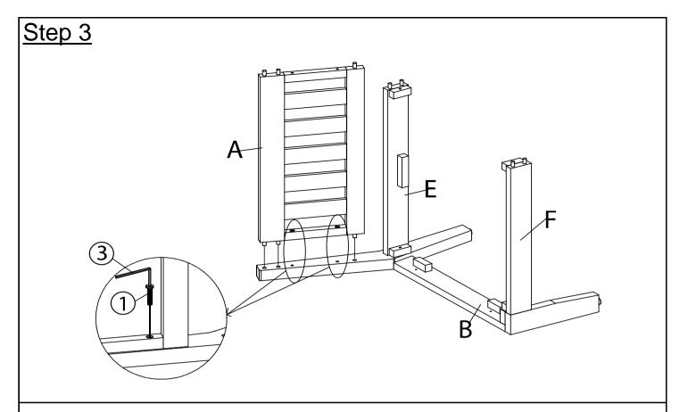
Insert dowels on Backrest Panel(A) into mountings on Left Panel(B). Attach Left Panel(B) to Backrest Panel(A) using Bolts( $\bigcirc$ 1) with Allen Key( $\bigcirc$ 3). **Do not fully tighten the Bolts.**
